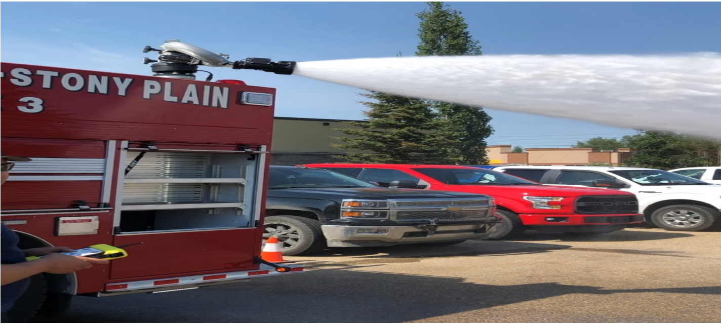
Pump Operator training with new Engine 3. The deck gun was relocated to a new location to provide better access for use to provide exposure protection.
