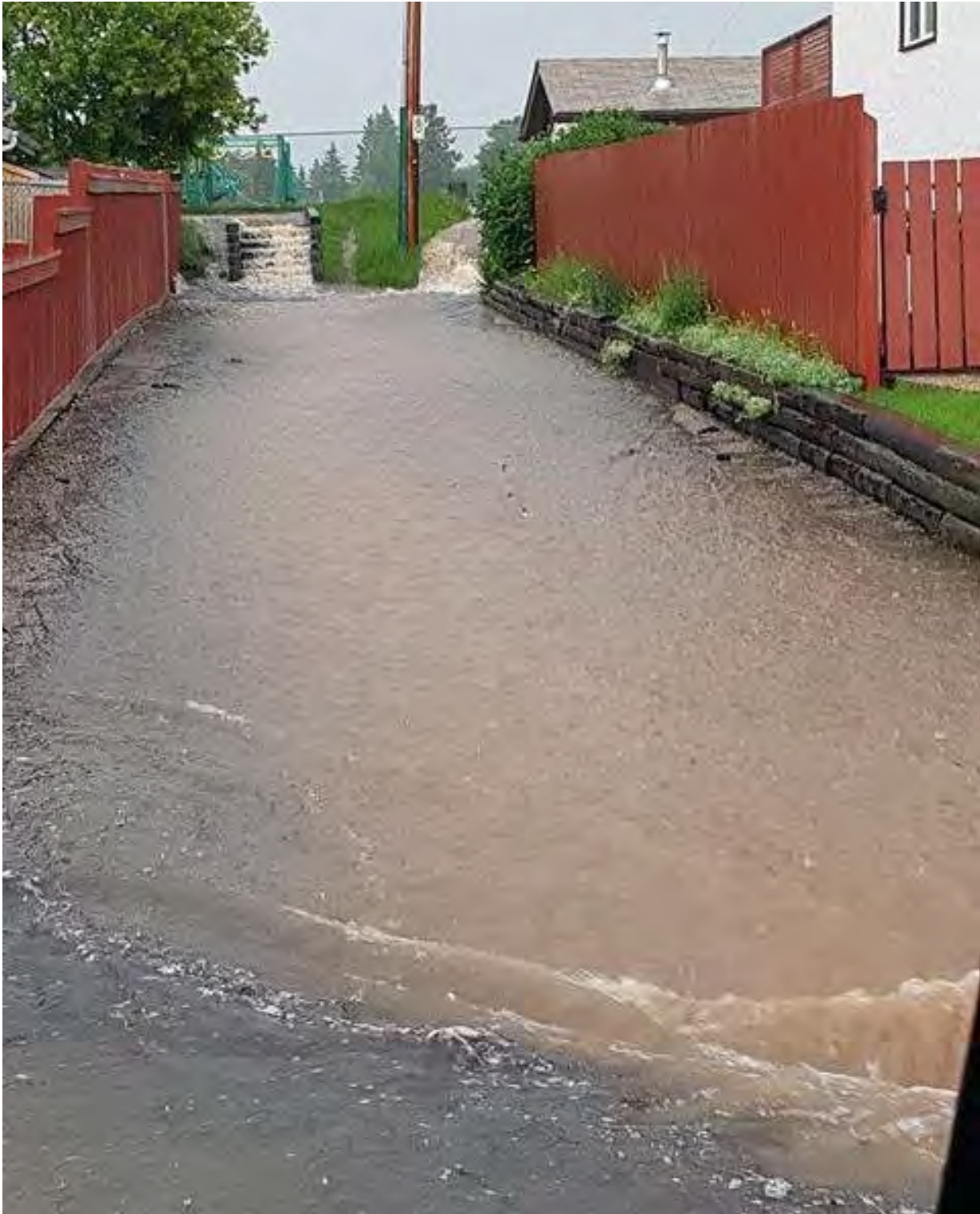
Figure D- 13: Area H – 57 Avenue just west of Glenwood Crescent, looking north in the alley and the school yard, showing significant amount of surface drainage flowing from the school yard towards 57 Avenue via the grass surface and the staircase. July 15, 2019
