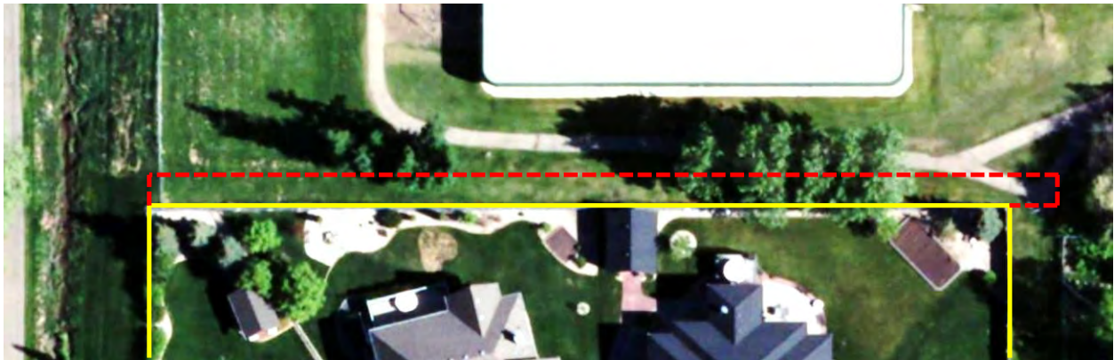
Figure 6-37: Conceptual Drainage Improvements for Whispering Cove North of Oatway Drive(yellow line is property line, red dashed line is proposed 3m easement on school property)
