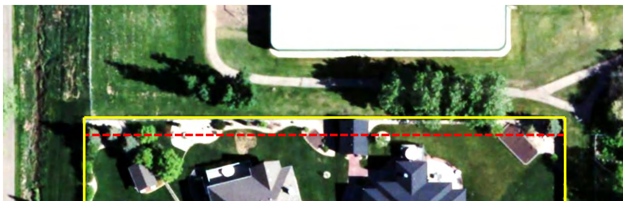
Figure 6-36: Local Drainage Concerns - Whispering Cove North of Oatway Drive – Air Photo showing Backyard Swale Area and Easement (yellow line is property line, red dashed line is 3m easement limit in property)
